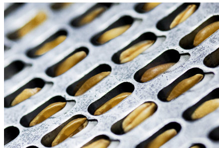
Kernels in pockets of the rotating cylinder.
