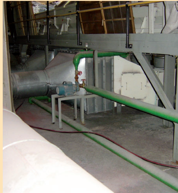
Radiators for indirect heating (heat source: hot water or steam)
